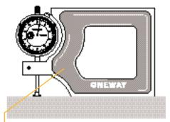
Loosen this screw and slide indicator down until needle is near top dead centre
